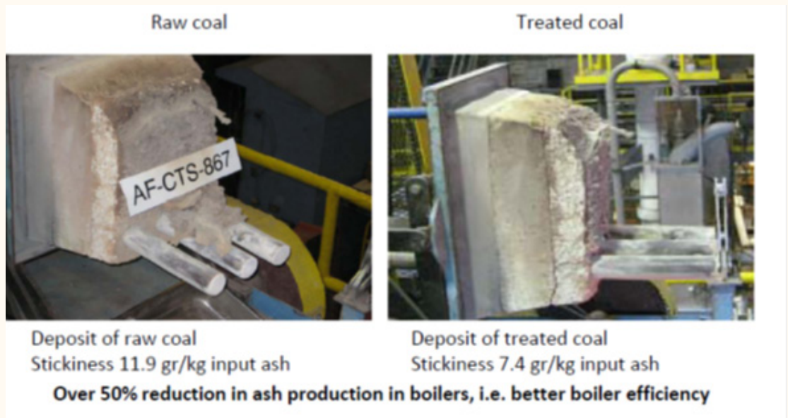
Figure 5. Over 50% reduction in ash production in boilers – better boiler efficiency. Source: MCI
